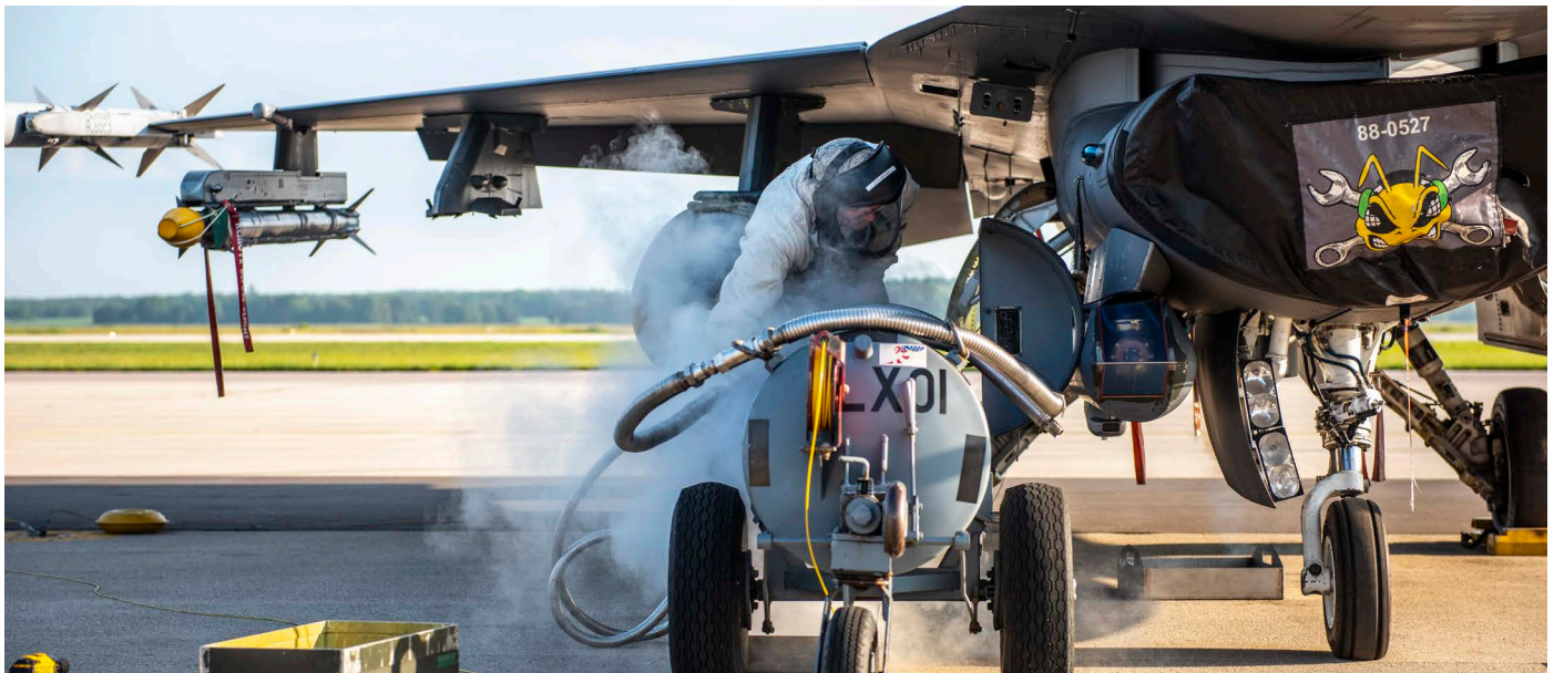
Staff Sgt. Austin Klein, 180 th Fighter Wing crew chief, services a liquid oxygen bottle for an F-16 Fighting Falcon during exercise Northern Lightning at Volk Field in Camp Douglas, WI. Northern Lightning is a joint training exercise emphasizing user-defined objectives resulting in tailored, scenario-based, full spectrum training. –Photo: U.S. Air National Guard photo by Airman 1 st Class Sarah Stalder Lundgren
