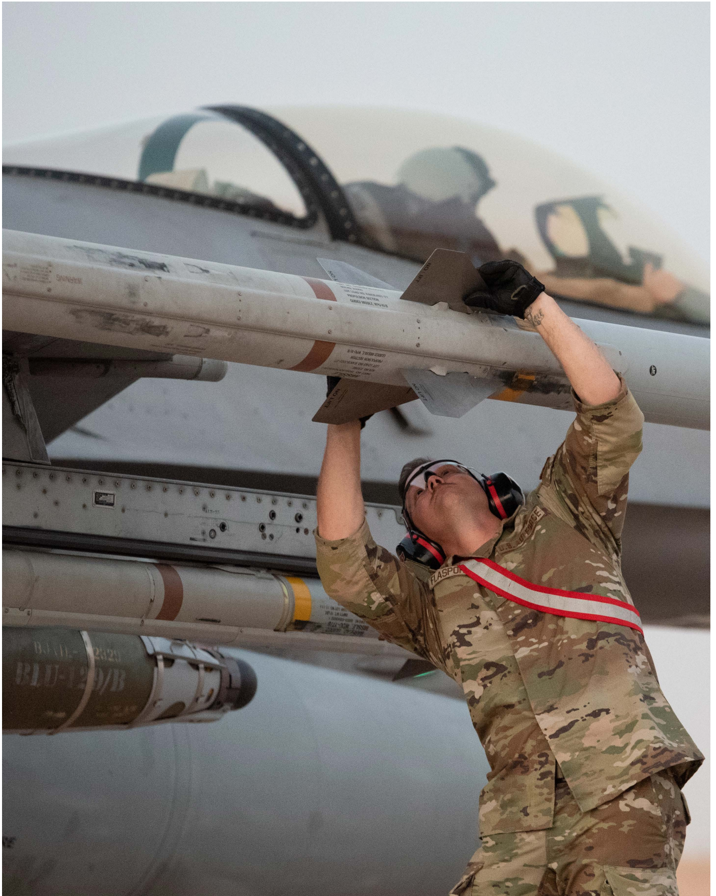
USAF Master Sgt. Dustin Flaspohler, 138 th Fighter Wing aircraft armament systems specialist, performs weapons checks on an F-16 Fighting Falcon assigned to the 125 th Expeditionary Fighter Squadron, after hot pit refueling at Prince Sultan Air Base, Saudi Arabia. Hot pit refueling occurs after an aircraft has landed and is still running its engine allowing for refueling in austere locations. —Photo: USAF photo by Tech. Sgt. Alexander Frank
